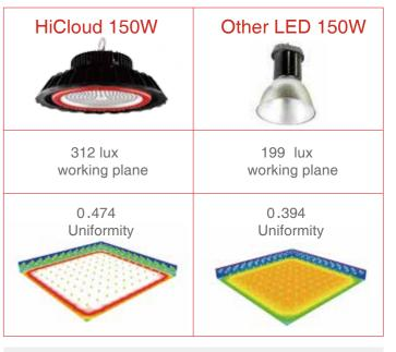
Room width 100m Room length 100m Room height 10m Fixture Qty 225pcs Fixture spacing 6.7m
